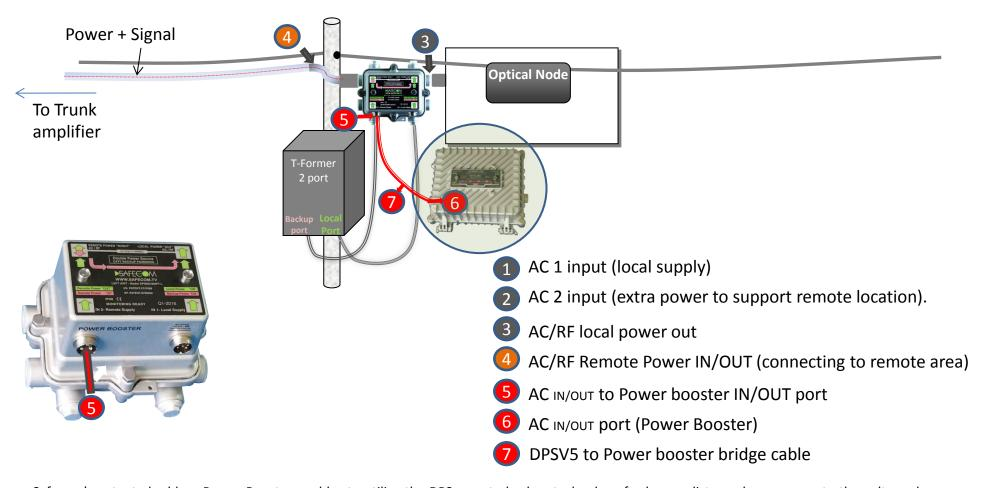
Safecom's patented add-on Power Booster enables to utilize the DPS remote backup technology for longer distance by compensate the voltage drop along the coax or electric cables.
